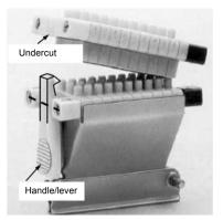
The plug block shown here is held together by a torsional snap element. The joint is exposed to rather low static mechanical loads. Since it must be possible to dismantle the push-in joint, the snap hook must be designed for frequent opening and closing operations. The components can be dismantled without any release force since the undercut of the snap joint is released by actuating a lever.
