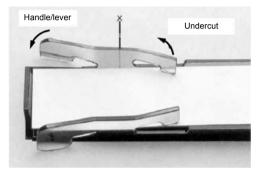
The writing panel made of polycarbonate (PC) constitutes nother example of a torsional snap joint. The arising mechan of loads are very low here as well since the snap element merely serves to fix the lettering. This joint is also designed former ent opening and closing.
